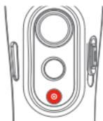
**Note: Single click during video recording allows taking a picture. You can tap the Bluetooth shutter release button during a single recording session as many times as you like to take multiple stills.**
