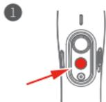
Click the function button five times. The motors will stop working. Status indicator turns solid blue.
