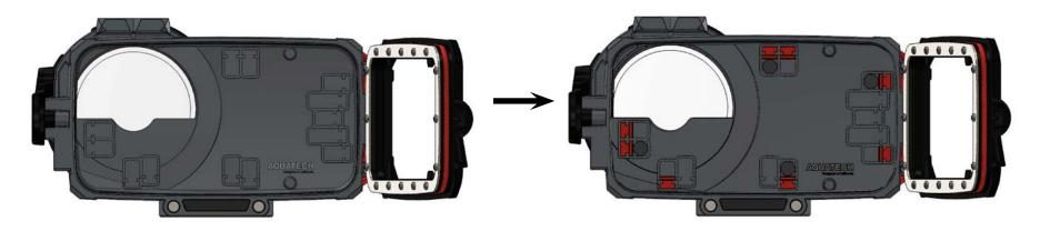
Install the included bumpers based on the bumper layout above.
