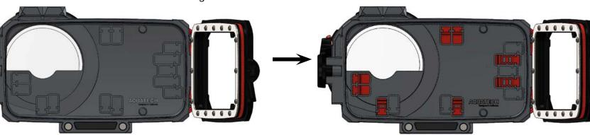
Install the included bumpers based on the bumper layout above.
